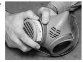
The inside probe tube must point below exhalation valve, see picture.
