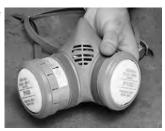
Check the inhalation diaphragms for dirt or damage and see that they are properly seated.
