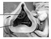
Check to see that the probed cartridge is seated properly, both inside and outside, and that it's flush against the facepiece.
