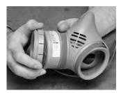
Place a new 8940 P100 Filter disk inside the retainer ring so that the side indicated is away from face. Replace the retainer ring.
