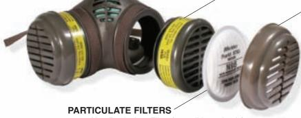
8910 N95 Particulate Filter (non-oil based only) 8970 R95 Particulate Filter (R95 For both oil & non-oil based particulates)
