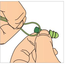
**TO ATTACH OPTIONAL CORD:** Form a loop at end of cord, position around groove at base of handle then pull down to lock in place.
