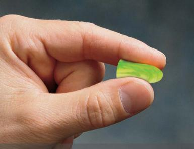
1. ROLL & COMPRESS. With clean hands, hold earplug between thumb and forefinger as shown. Roll and progressively compress the entire tapered end of the earplug to a small wrinkle-free cylinder.
